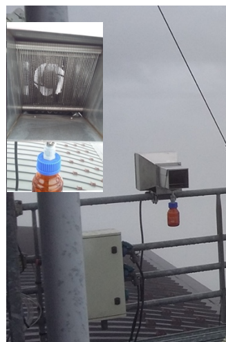
Figure S2. Left: Construction of the CASC2 sampler: 1 = ventilator fan; 2 = strands; 3 = inlet; 4 = flow straightener; 5 = sample drainage. Right: CASC2 installed at PUY. Picture : M. Vaitilingom.
